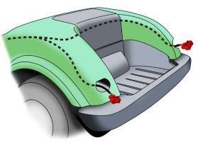
6. Make sure the taillight leads reach the holes in the rear body. Once the leads are in position, use cable ties to loosely secure the harness in place and away from any moving parts or areas where it can be pinched. Holes can be drilled in the rear fenders if needed for wire ties.
