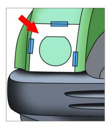
INSIDE of the marked area. Test fit the taillight and make any adjustments before removing the tape. Once the light fits, remove tape and sand any rough edges.
