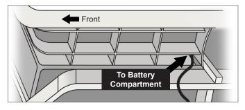
4. Make sure the battery leads can reach the appropriate terminals. Set the leads aside and away from the terminals.
