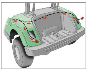
behind the battery compartment and over the passenger side wheel well.
