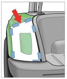
light fits, remove the tape and sand any rough edges.
