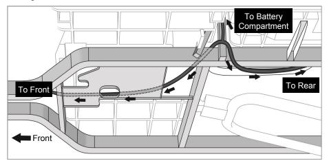
Feed the rear portion of the harness through the cart so the taillight connections reach the holes in the rear body. The harness can be run parallel with the cart's harness for a cleaner installation.
