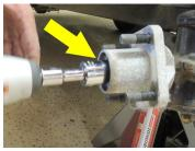
10. Disconnect the tie-rod ends from the spindles by removing the safety pin and the crown nut on the tie rod end. Use a tie rod fork to dislodge and remove the tie rod ends from the spindles. Retain hardware.
